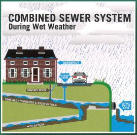
Combined sewer systems are designed to collect stormwater, sanitary sewage and industrial wastewater in the same pipe. In dry weather, combined sewer systems transport this flow to ALCOSAN for treatment. During heavy rain or snow melt, however, the wastewater volume is too great and the excess flows into our local waterways. These are called Combined Sewer Overflows (CSOs).
